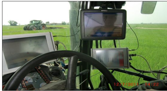
Figure 3. The tractor's cab full of monitors and cables, due to the lack of communication between monitors and sensors of different brands
