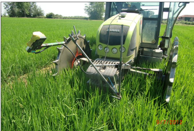
Figure 1. The articulated mechanic support of the vigor sensor, to compare the different responses at three inclinations, with best result when inclined 16° from the horizontal.
